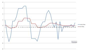
Fig 3. Comparing the signal with and without weighted moving average filter over time. The blue line shows the acceleration signal on the z-axis while writing the letter a without any filter applied. The red line shows the same signal for the very same movement with the filter applied.
