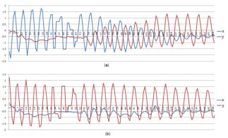
Fig 5. Comparing the acceleration data before and after applying the rotation of the frame of reference while the device is moving up and down repeatedly and rotating around z-axis 90 degrees; a) acceleration without applying the rotation on the frame of reference; b) acceleration after applying the rotation on the frame of reference.
